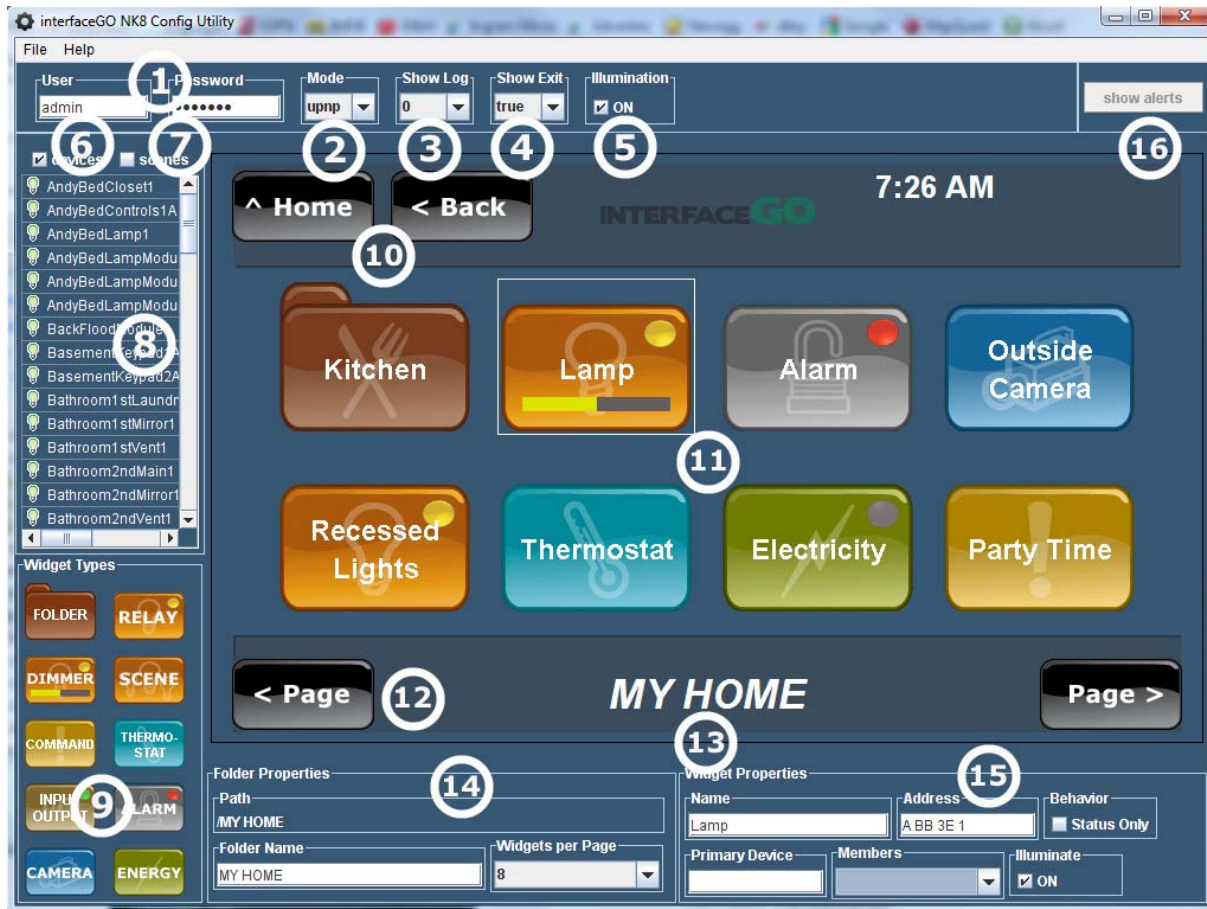
The interfaceGO NK8 Config Utility
