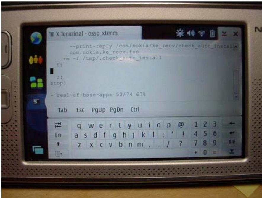
Once the cursor is in the correct location, hit the on-screen ESC button, then type the following command to put the editor into "insert mode":
